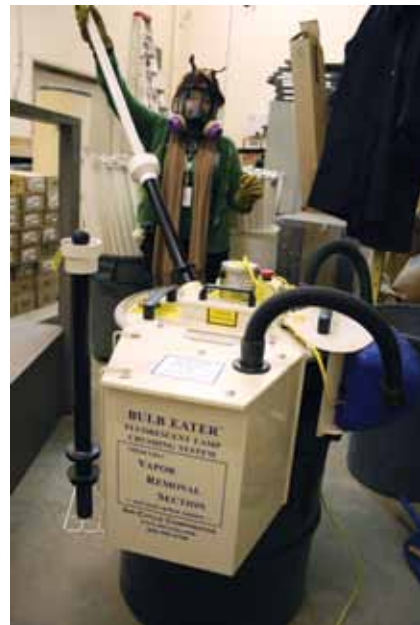
As part of the Campus Lighting Retrofit, a bulb eater crushes outdated fluorescent tubes and isolates the mercury vapour, which is safely removed and transported to a hazardous waste facility. The crushed glass and aluminum are recycled.
