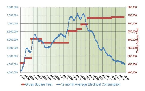
These significant reductions have been achieved through intentional development and utilization of the campus computerized energy management system, tight scheduling of occupied spaces, lighting and mechanical upgrades, daylight controls and temperature setbacks. Another factor in the reductions, which is difficult to measure, is increased awareness of environmental sustainability and resulting behavior change in the campus community.
