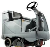
The Advance AquaRide is equipped with a patented AXP onboard detergent dispensing system. The AXP system eliminates pre-mixing of detergent and water because the two are stored separately in the machine until the solution is sprayed on the scrub head. This prevents solution waste and increases cleaning productivity by eliminating the need to
