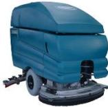
The tenant auto-scrubber can clean scrub and mop floors at once. It can also be used for water extraction on open areas. It is battery operated with the main scrubbing system on the front. Water jets supply the water with the cleaning solution at an even rate while a squeegee mounted on the back collects all the water and directs it to a vacuum. Floors are virtually dry in a couple of minutes. Rubber bumpers and non-marking tires protect facilities.
